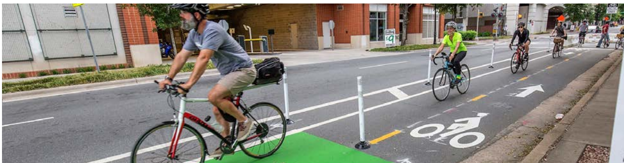
A separated bicycle lane in Uptown Charlotte, NC.
